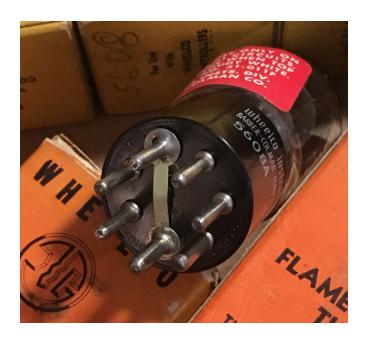
One very important note about the 5608. It has come to our attention that certain 5608 labeled "Flameatrol" have had a external straps applied between two pins. You must disconnect this strap by either unsoldering it or cutting it out with nippers or snips before use in the EMIA Amplifier.
