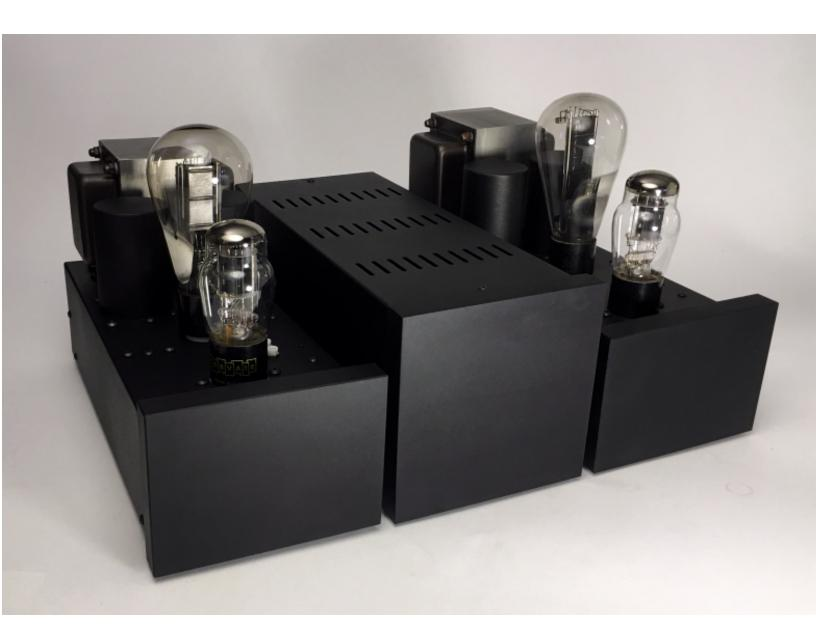
The EMIA Permalloy Amplifier is an all-triode, two-stage, transformer-coupled, single-ended amplifier comprising three chassis. Each side chassis contains the last stage of the high voltage filter, the filament regulation, and the entire signal amplification circuit. The shared center chassis contains the the power transformers and first filter stages for both driver and output stage high voltage as well as both driver and output filament supplies.
