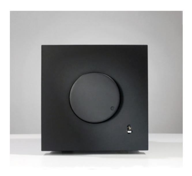
The EMIA Elmaformer is a stereo volume control based on multiple tapped auto-transformers. The unit has 47 steps of 1.25dB each. The complete gain range is from -51.25 to +5dB. As the name implies, the switch is our favorite high quality unit from Elma of Switzerland. The cores of the auto-transformers are made of 80% Nickel, also known by its trade name of Permalloy. Each auto-transformer uses non-magnetic brass channels for that last bit of signal circuit preservation.
