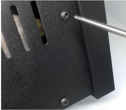
To access the tubes, use a 2mm hex driver to remove the 10 button-head screws on the appropriate chassis. Gently slide the cover back and then up and set it to the side. The tubes and sockets are now exposed.
