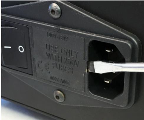
The fuse holder is in the middle of the IEC inlet. It is accessed with a small flat blade screwdriver. The holder has dual voltage designations on it and can be rotated 180° and installed to change from 100-120V to 200-240V to match your line voltage.
